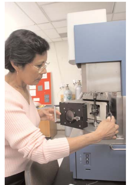
Researcher places a sample on the DMA to measure glass transition temperature ( T_g )
