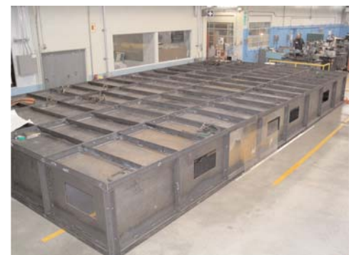
New 16' by 32' table for Phase IV investigation of wider roofing membranes
