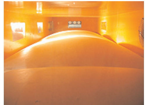
Dynamic wind gusts over a mechanically attached single ply roofing system
