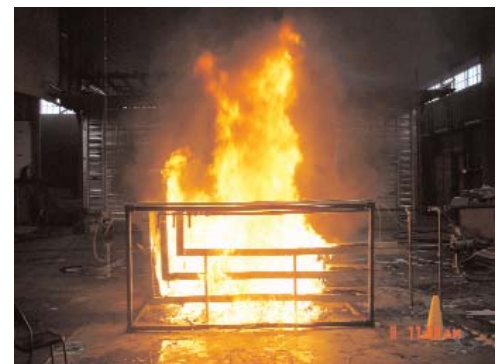
A cable tray fire
