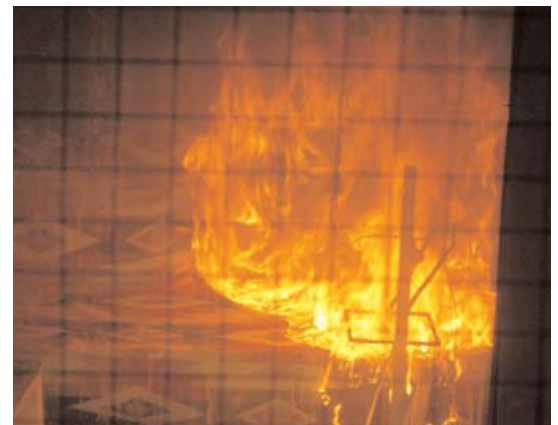
Fire spreading on a sofa before CAF activation
