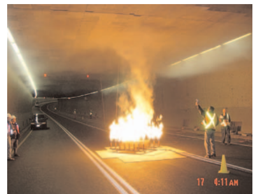
Full-scale fire tunnel test
