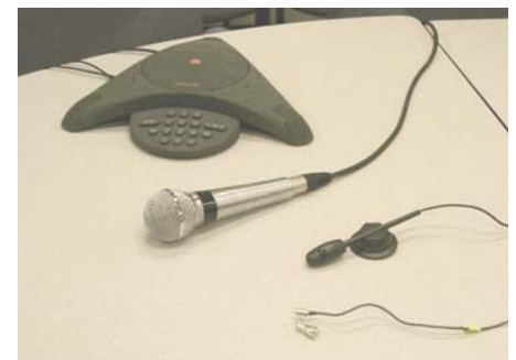
Examples of several devices commonly used for speech pickup in rooms (from top): hands-free conference phone, public-address microphone, computer microphone, clip-on lavalier microphone.
