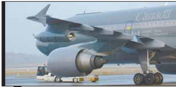
The CC-150 Polaris Multi Role Transport Tanker aircraft at 8 Wing Trenton. Air-to-air refuelling pods can be seen just inboard of each wingtip.
