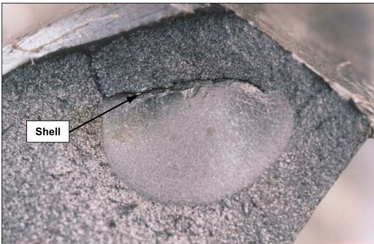
Photo 2. Close-up of detail fracture
