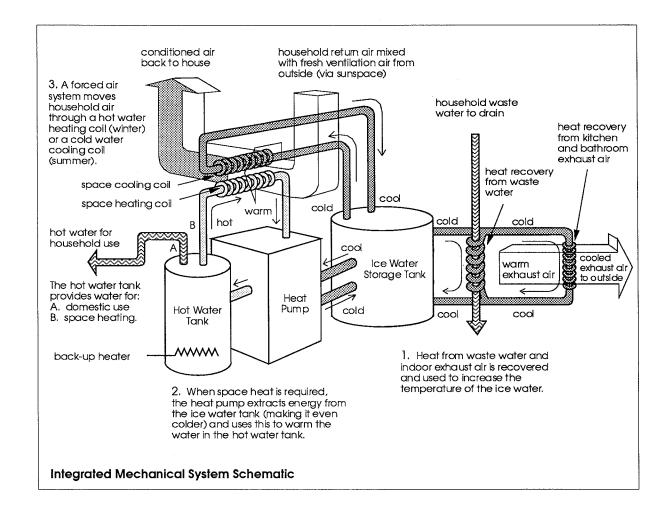
provided by directing the household return air over a cooling coil that is connected to the ice water storage tank.
