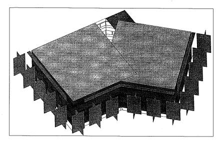
Above: A rendition of the Kamloops office building design as seen by the DOE2.1E simulation program. The strange shapes are the program's way of representing trees, which in this case provided a considerable reduction in summer cooling loads.
