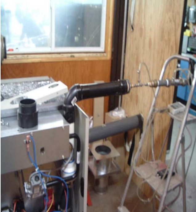
Figure 18 – Heating Module Leakage Test Set-up Sample No. 04-06-M278-5
