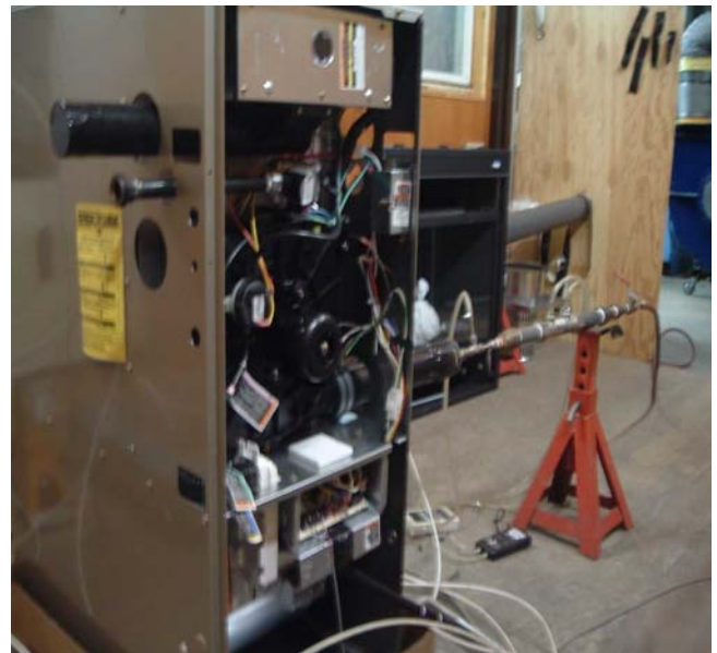
Figure 19 – Heating Module Leakage Test Set-up Sample No. 04-06-M278-6
