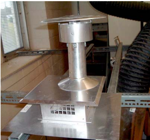
Figure 12 – Fireplace Insert Vent Termination Sample No. 04-06-M0278-7
