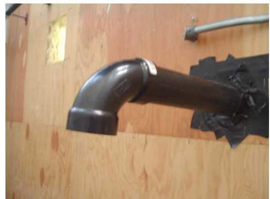
Figure 2 – Exhaust Vent Termination Sample No. 04-06-M0278-1
