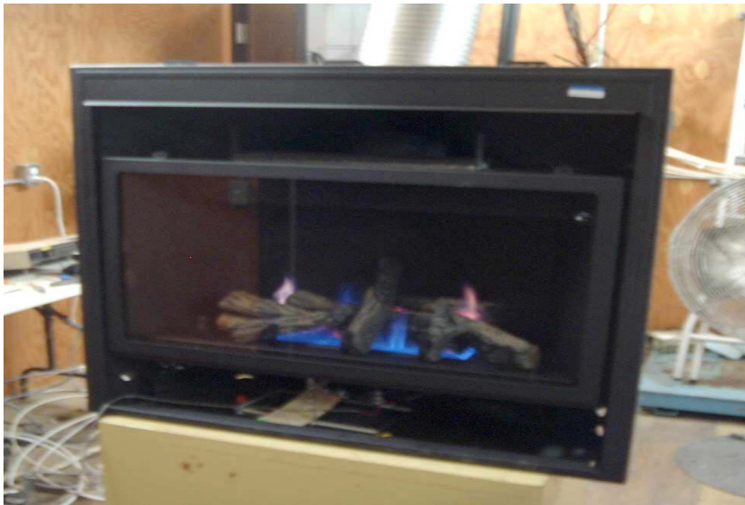
Figure 14 –Zero Clearance Fireplace In Operation Sample No. 04-06-M0278-8
