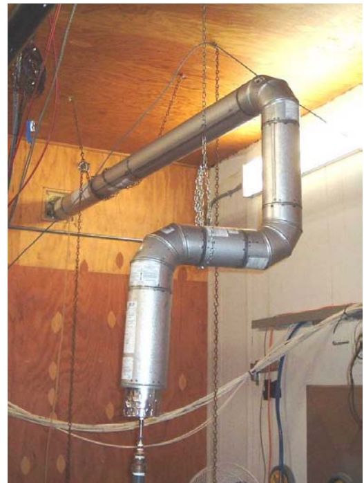
Figure 17 – Static Leakage Test Set-up ‘Type B’ Vent System Sample No. 04-06-M0278-2
