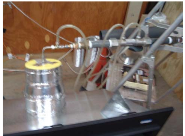
Figure 21 – Heating Module Leakage Test Set-up Sample No. 04-06-M278-8
