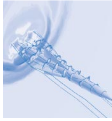
Simulation of body and wing vortices on a missile using computational fluid dynamics
