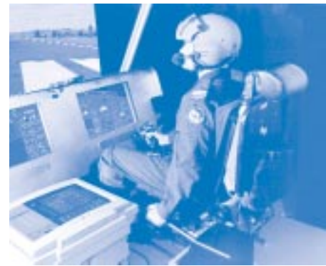
The Aircrew Cockpit Demonstrator enables virtual prototyping of cockpit instrumentation for human factors assessments
