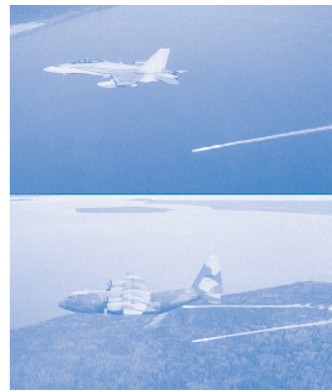
Pyrophoric decoy flares have been developed to protect the CF-18 and CC-130 from IR seeking missiles
