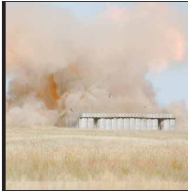
DRDC-Suffield's full-scale, destructive testing of the HESCO ISO-Bunker.
