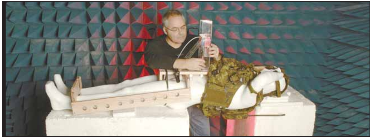
DRDC-Ottawa technologist Alan Walsh sets up a test that will measure how much RF energy would be absorbed in the body of a soldier wearing the WES Player Unit Radio in a training exercise.
