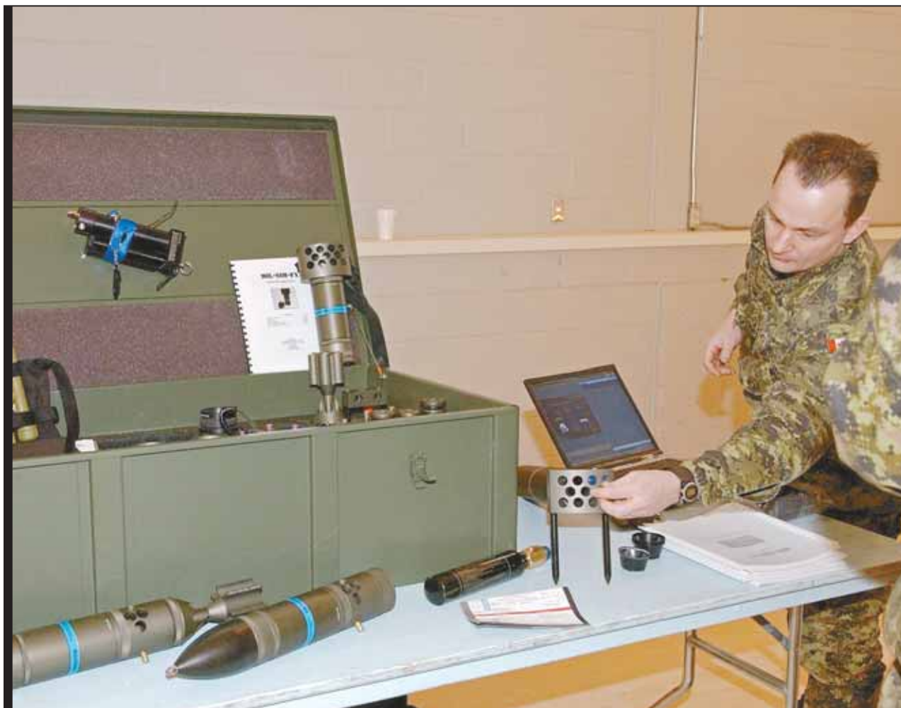
Capt Philip Meaney adjusts the paintball dispenser on a Claymore simulator. The improvised explosive device simulation kit has a wide variety of devices for adding realism to training.
