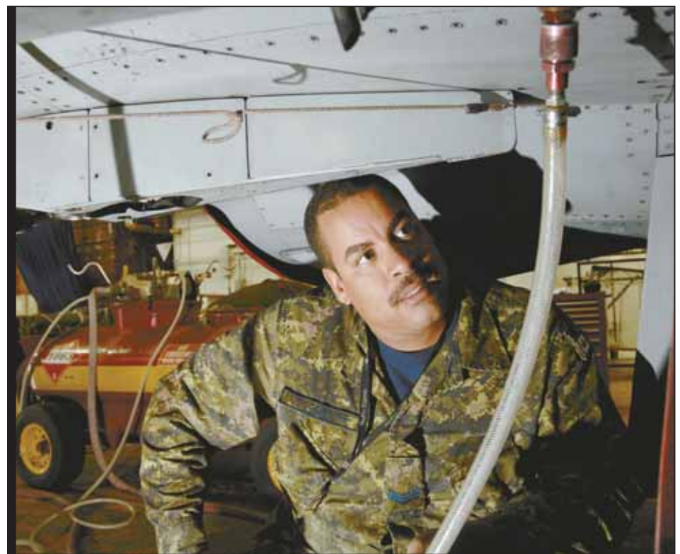
Cpl Ian Rickman, an aviation technician with the snag crew at 441 TFS, defuels a CF-18. Technicians are critical to exercises like Ex MAPLE FLAG.
