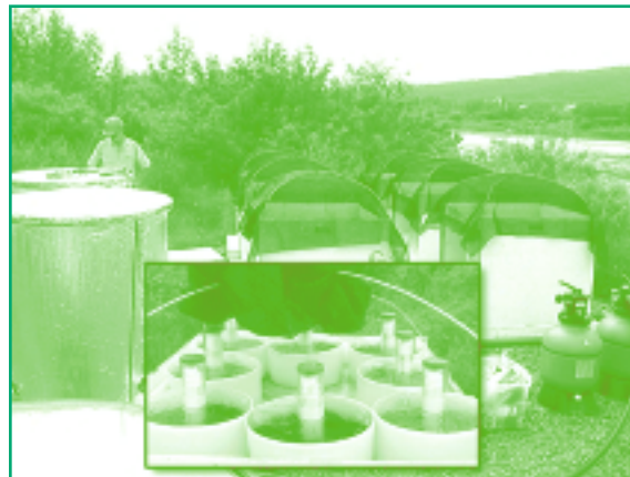
Field-based artificial stream system used for assessing the ecological effects of effluents on riverine ecosystems.
