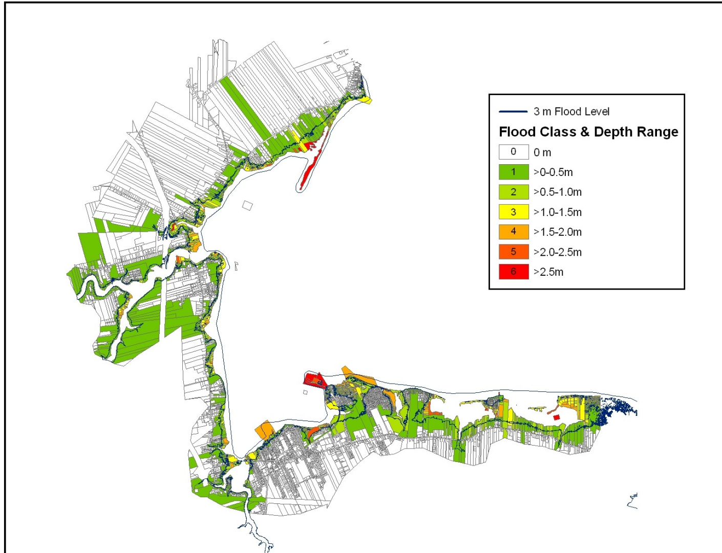
Figure 4. Flood risk to properties, 3.0 m above DEM datum water level, existing structures. The blue line represents the maximum flood limit during the January 21, 2000, storm-surge event.
