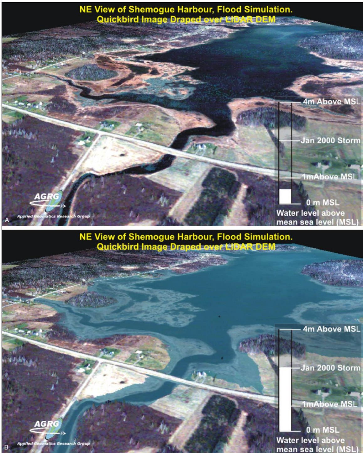
Figure 10. Example of flood-risk map visualization. A. Quickbird satellite true colour image draped over LiDAR DSM, normal water level within the tidal range. B. Simulated water level associated with the January 2000 storm-surge event. Includes material (2004) © DigitalGlobe, Inc. all rights reserved.
