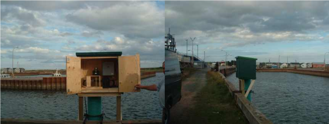
Figure 1. Tide-gauge hut, tide-gauge recorder and logger at the Wood Islands site. Photograph kindly provided by Fred Carmichael (CHS).
