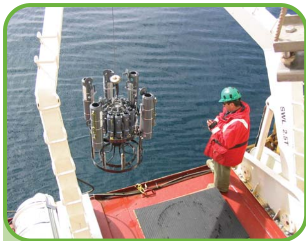
A rosette sampler is used to record temperature and salinity, and to collect water samples at different depths in the water column.
