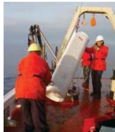
Recovering a sediment trap from the waters of the Bras d'Or Lakes. The trap has been moored upright beneath the water surface for about six months. The small bottles visible at the bottom of the trap contain samples of the particles falling through the water collected during pre-programmed intervals.
