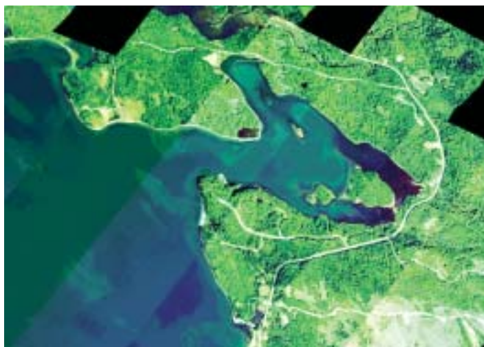
Compact Airborne Spectral Imager (CASI) image of a small portion of the Bras d'Or Lakes showing delineation of underwater features in depths of 5-10 m. These features will be associated with benthic habitat types through ground truth studies and comparison with multibeam sonar data.
