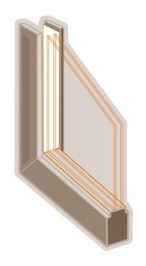
If you have central air conditioning and keep some windows closed year-round, leave storm windows on these as well. The air space between the two windows provides extra insulation and helps keep the house at the temperature you want.
