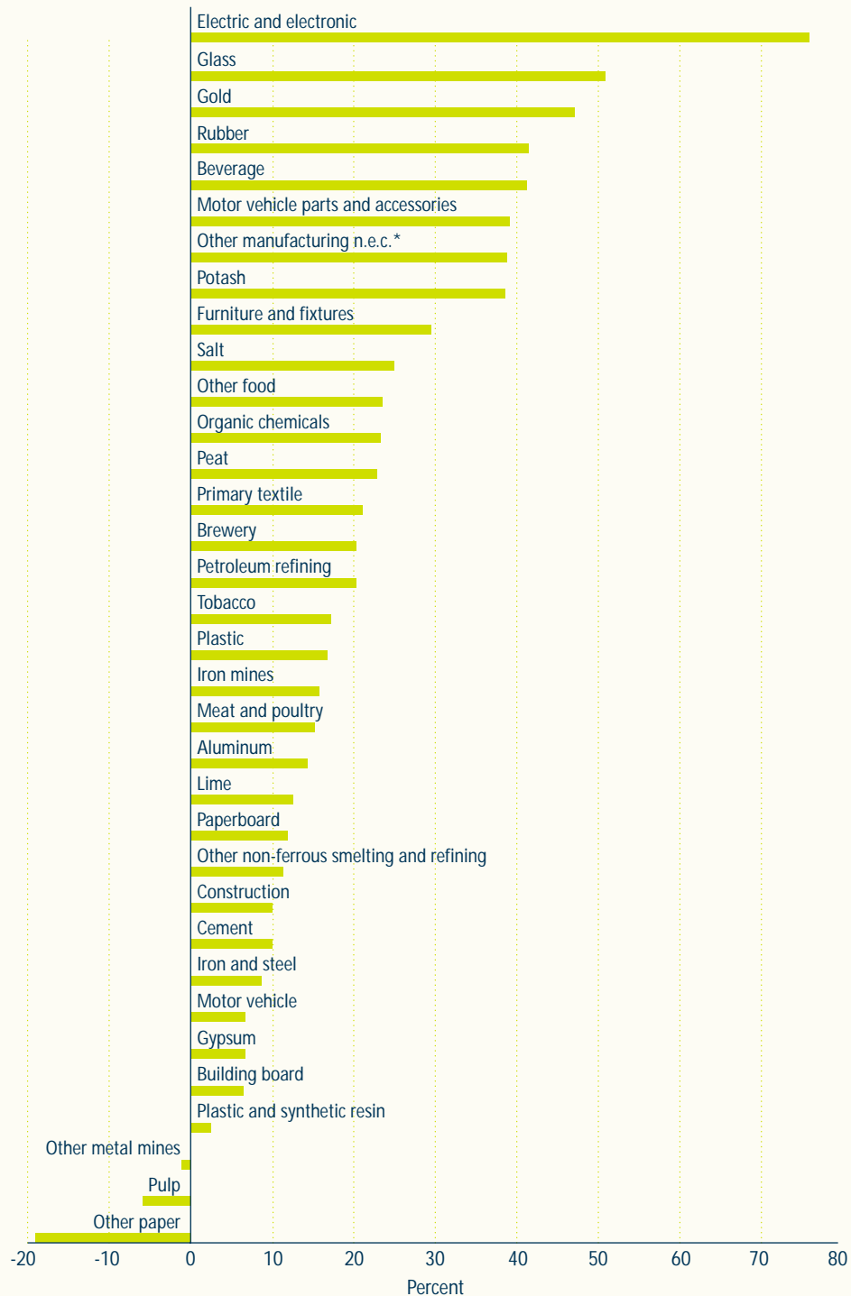
FIGURE 31 Reduction in Energy Use per Unit of Output for Selected Industries, 1990 to 2000
