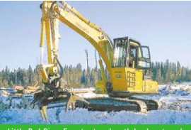
Little Red River Forestry tree length loader at work
