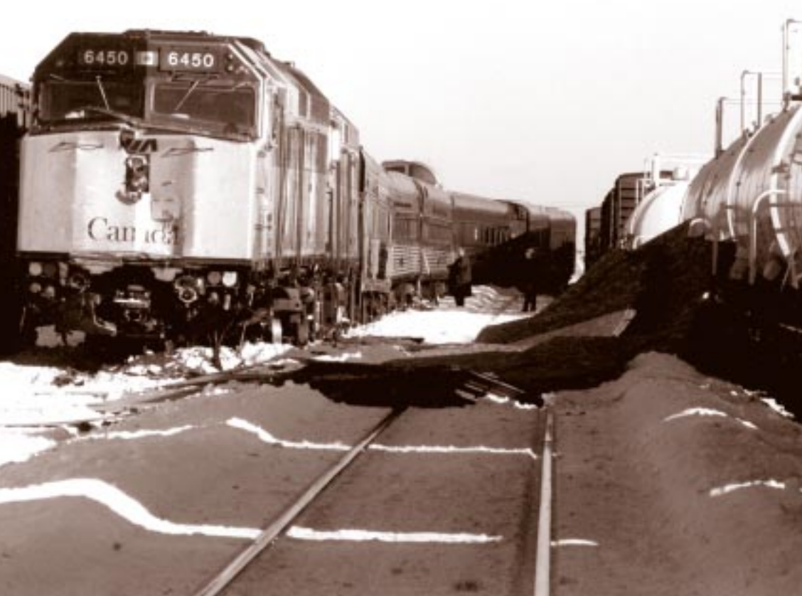
Some of the damage to lead locomotive VIA 6450. Note displaced front truck under centre of locomotive (which damaged the battery boxes and diesel fuel tank) and impact marks on collision posts on the front of the locomotive. (Source: Miramichi Leader newspaper)
