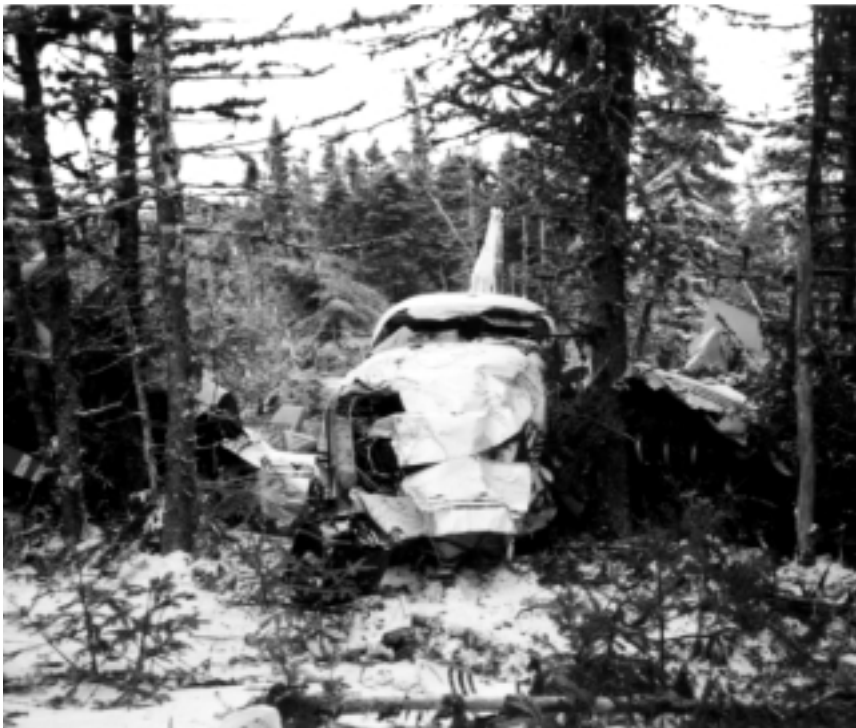
The pilot of this Aztec had little experience with flight in icing conditions and was surprised at the amount of icing and its effects.
