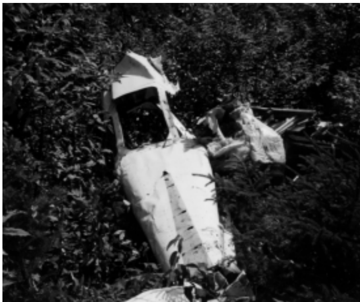
The pilot of this Cessna 210 tried to squeeze between thunderstorms, but the aircraft broke up in midair.
