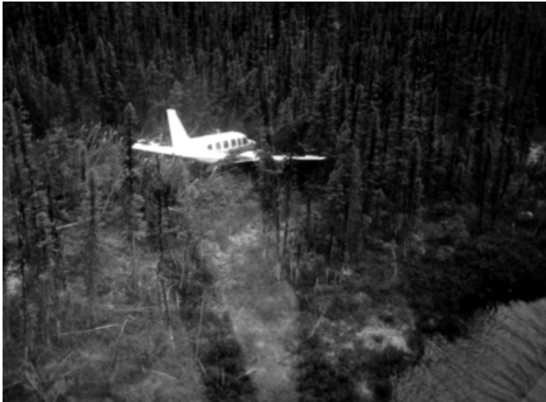
The Navajo pilot did not believe what the fuel gauges were telling him, and the fuel tanks ran dry.
