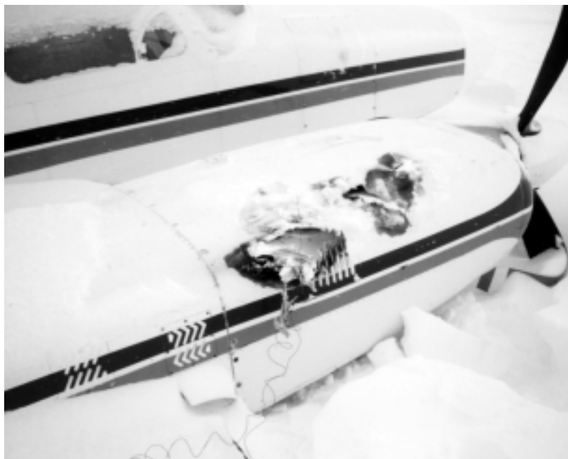
Modifications to the cabin heating unit that were not done "by the book" led to an engine fire on take-off.
