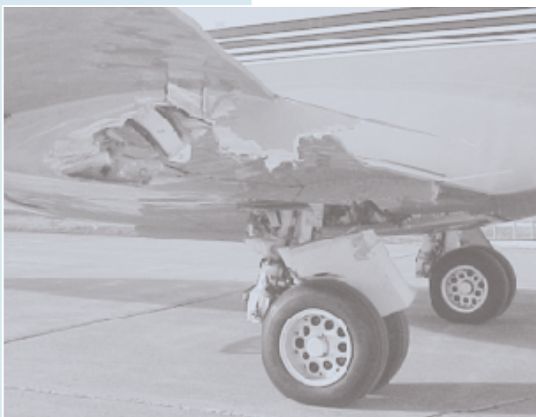
Damage to an Astra SPX, which struck treetops on approach to Fox Harbour, Nova Scotia, in March 2000.
