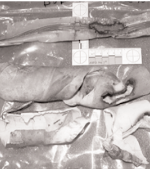
Contaminated thermal-insulation blankets such as these pose considerable fire hazards.
