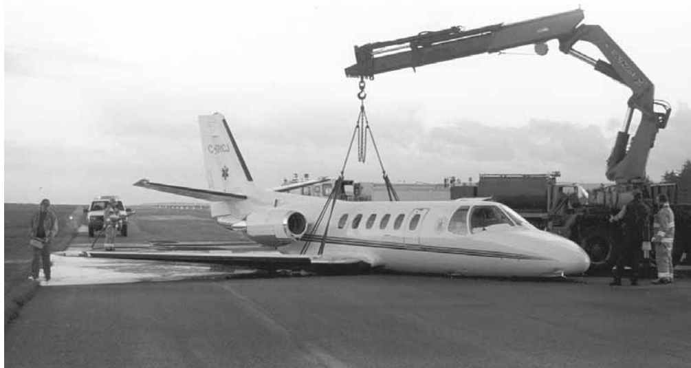
The Citation is raised so that the landing gear can be extended.
