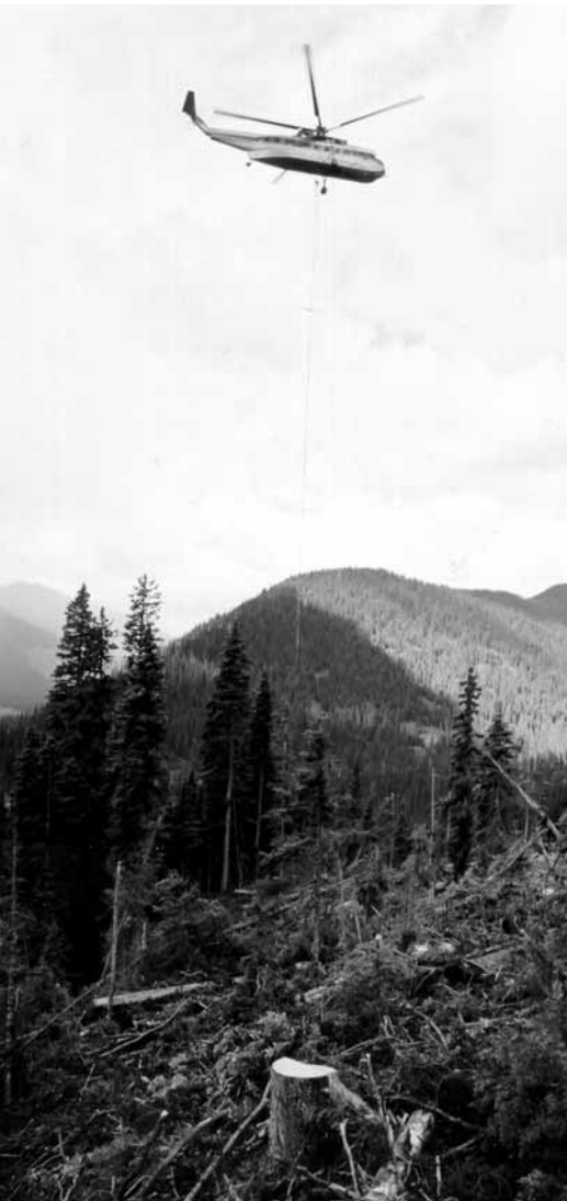
Sikorsky S-61 using a longline to pick up logs
