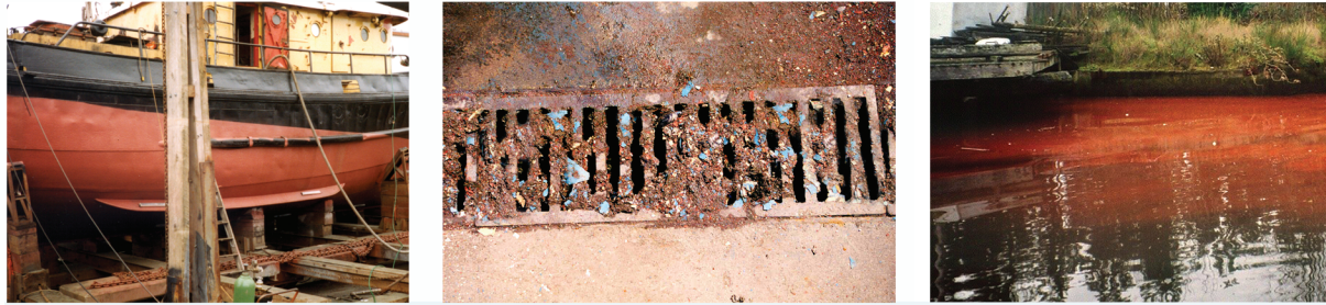
Lack of proper containment during antifouling paint removal can result in deleterious substances being released into the aquatic environment.
