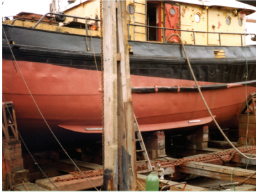
Lack of proper containment during antifouling paint removal can result in deleterious substances being released into the aquatic environment.
