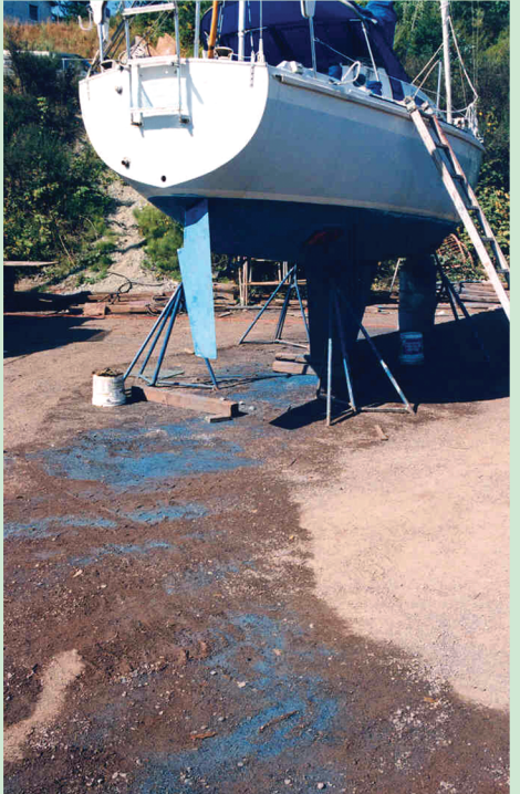
Paint chips and residue not properly contained may flow into fish bearing waters, resulting in a violation of the Fisheries Act.
