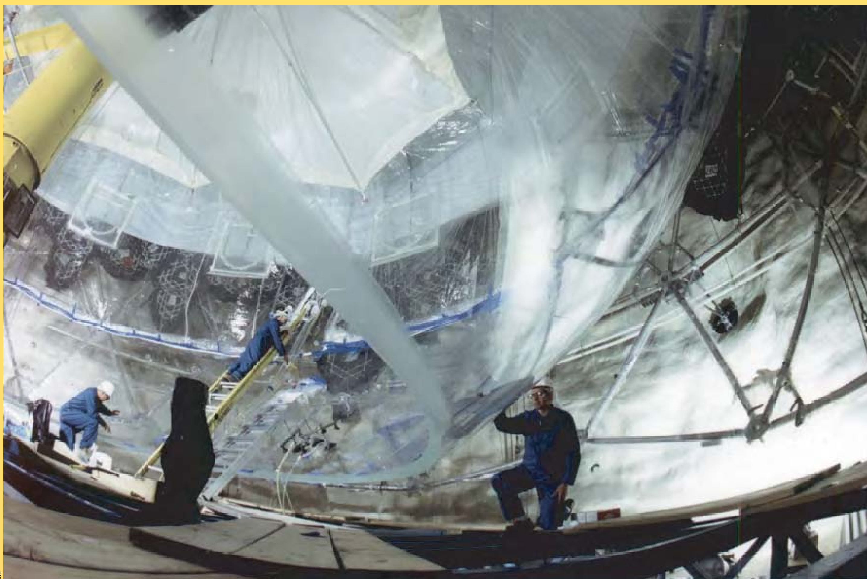
The acrylic vessel, built to hold the heavy water which is essential to the experiment, is being inspected.
