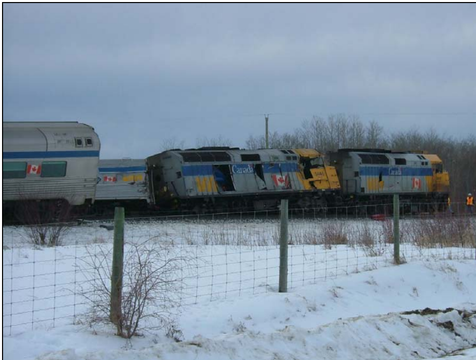
Photo 3. View of the damage to the north side of the two locomotives
