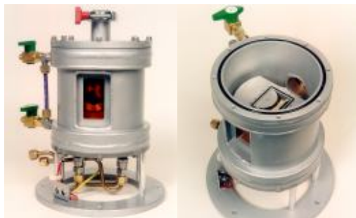
Figure 3: Full elevation and partial top view of neutron or x-ray sample holder capable of achieving humidities approaching 100%.
