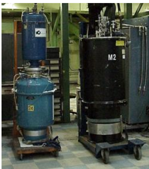
Figure 1: The 7 Tesla vertical and 2.5T horizontal field magnets. Both pieces of equipment can be mounted on our triple axis spectrometers.
