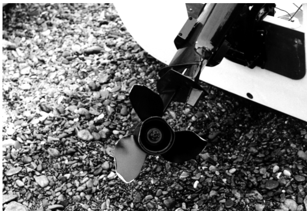
Photo 3. View of damaged propeller blades
