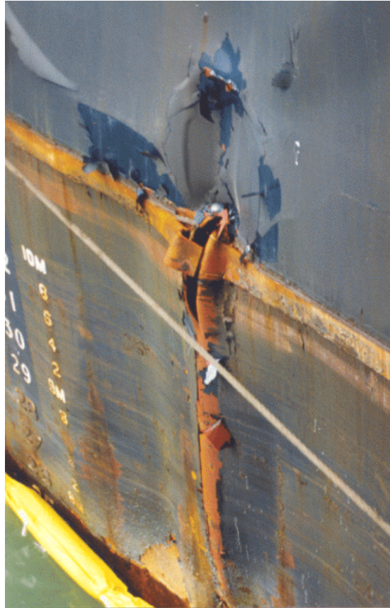
Photograph 3. Buckling and fractures on the port side
