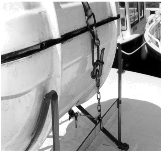
Photo 13 Manual release Senhouse slip securing inflatable liferaft in cradle on superstructure top.
