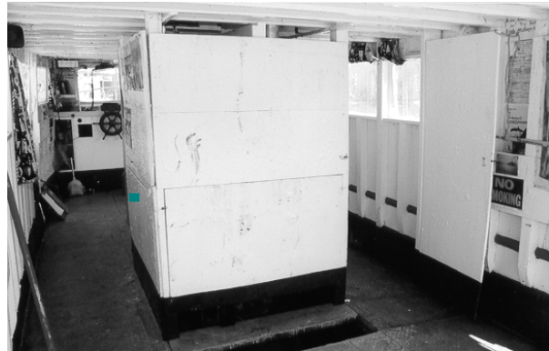
Photo 5 Engine casing with portable plywood panels in place showing opening at aft end for engine ventilation.
