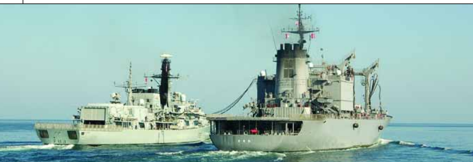
A Royal Navy Frigate refuelling from a Japanese Defence Force AOR: The utility of working with allies. (Photo Credit: MCpl Colin Kelley, Formation Imaging Services Halifax)
