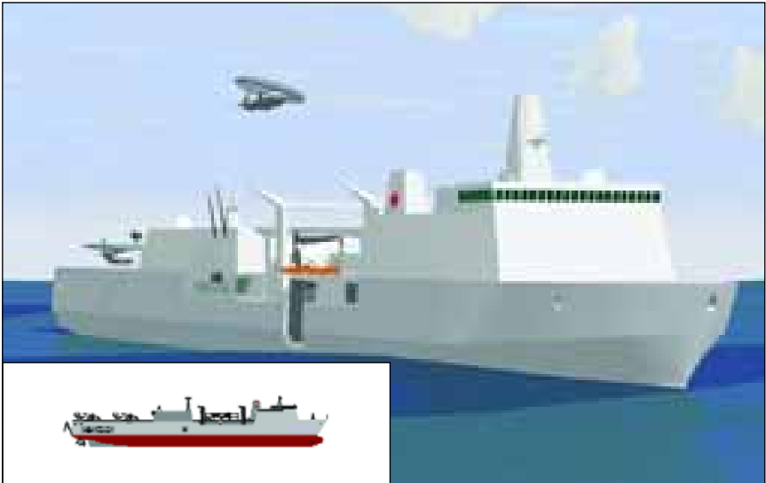
The proposed Joint Support Ship — capable of refueling, Task Group Command, troop transport, medical support and disaster relief
