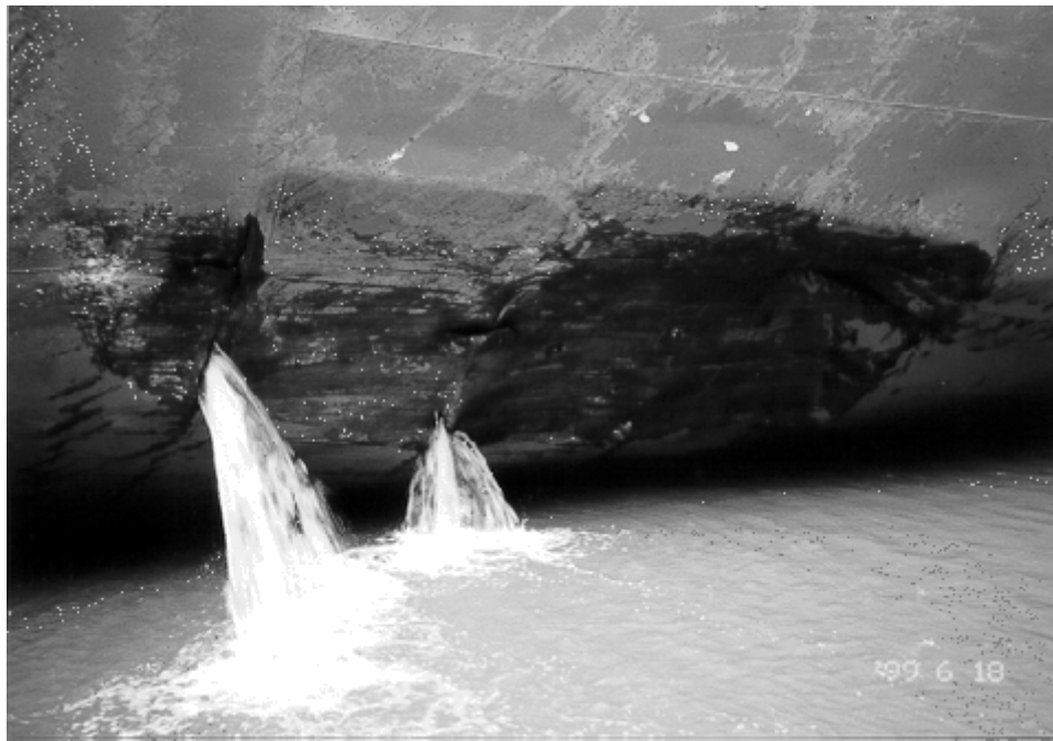
Photo 4 Hull damage caused by grounding
