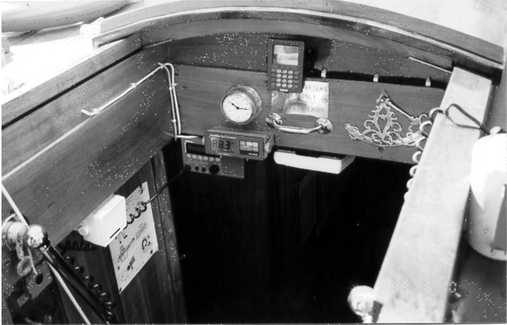
Depth sounder repeater (under clock), with taped instructions to add 10 (feet). Soundings indicated in feet.
