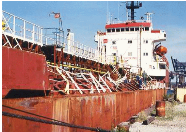
Photo 3. Port-side damage to Coral Trader
