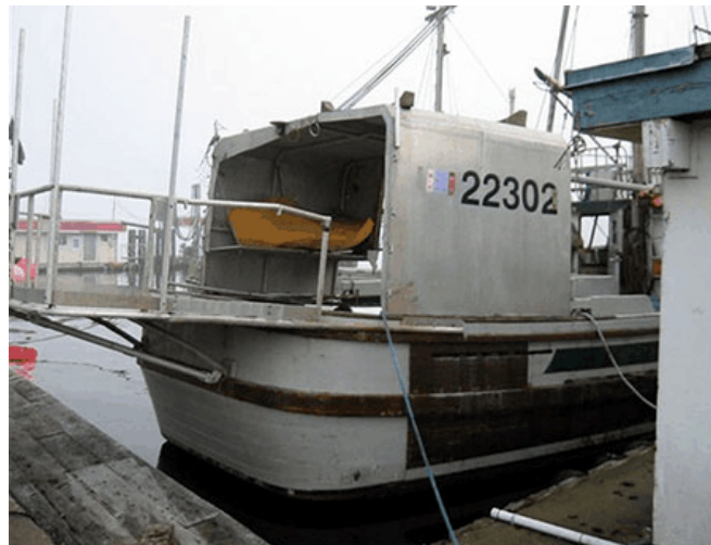
Photo 5. Stern view of double extension platform and baiting enclosure
