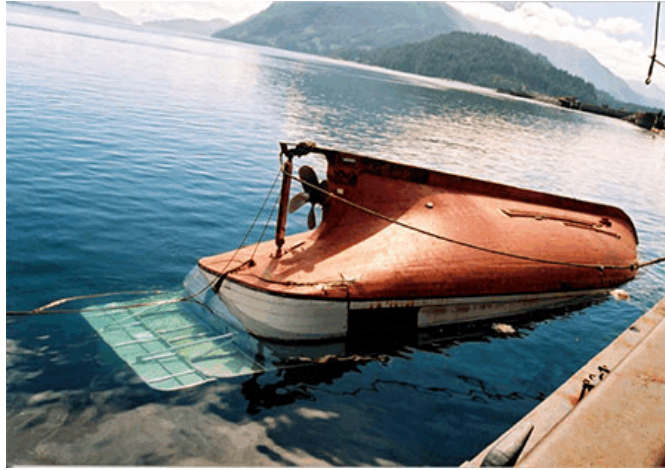
Photo 3. Capsized Fritzi-Ann alongside wharf, showing submerged deck extensions
