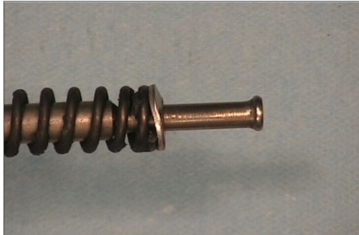
Figure 1 - Spring and bent spring retainer washer on the rod section of occurrence RH nosewheel steering tube assembly
