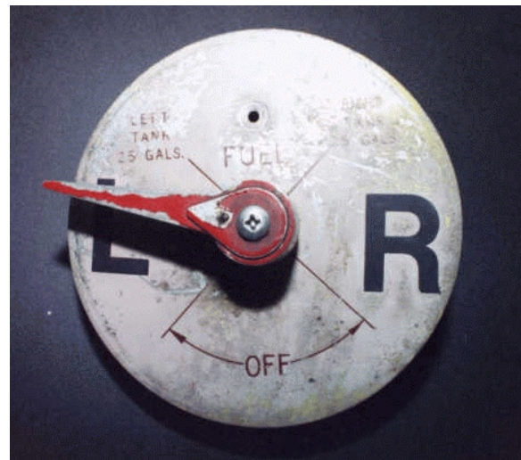
Figure 2 – Fuel selector over L, not in detent
