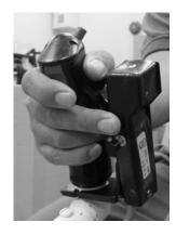
hands could easily access the dump switch while maintaining a normal grip on the cyclic.
