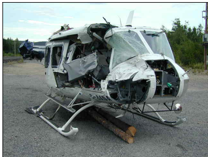
Photo 1. Damage to Bell 205 A-1, C-GADA
