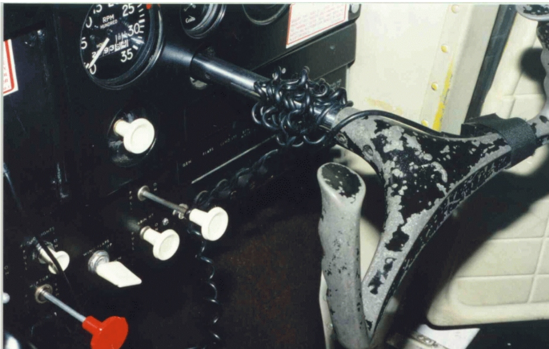
Figure 2 - The right control column movement probably was restricted by the push-to-talk cord, which snagged on the cabin air control knob.
