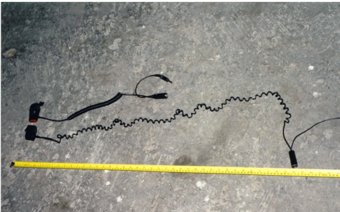
Figure 1 - Top: left push-to-talk cord (new). Bottom: right push-to-talk cord (old).
