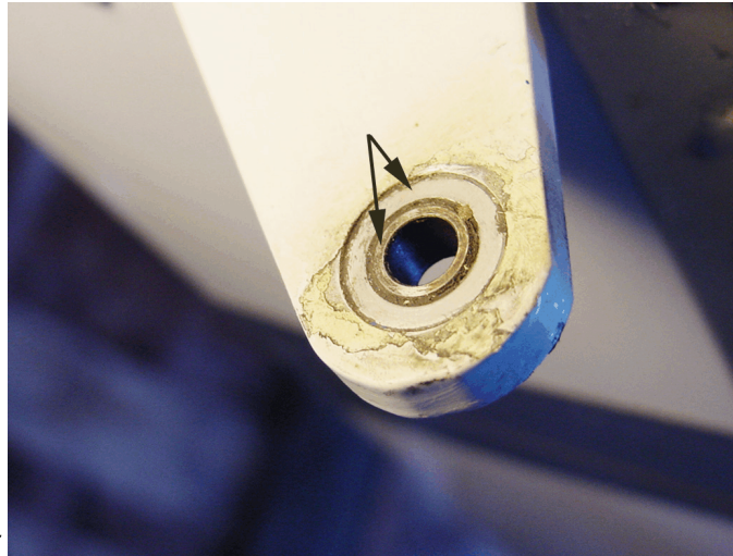
Photo 2. Inner and outer bushing arrangement
