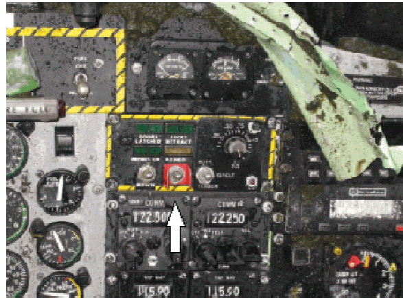
Photo 2. System indicating lights and door armed switch (indicated by white arrow) in the On position
