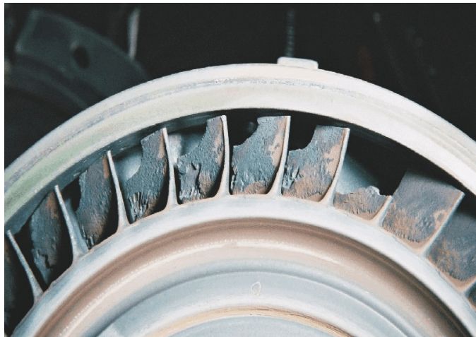
Photo 1. Sulfidation of number 1 GP turbine
