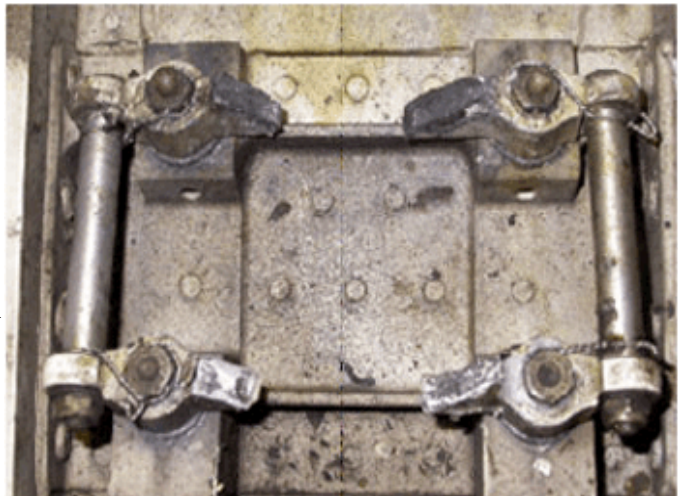
Photo 2. Upper and lower attachments on aft bulkhead
